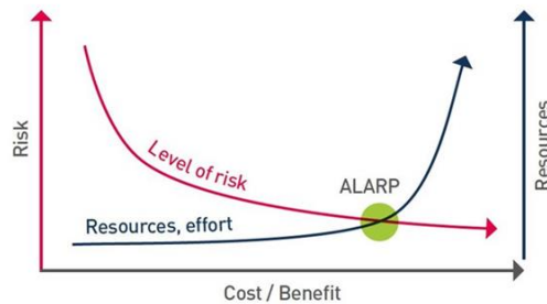
Figure 1 ICMM 2021's Concept of assessing benefit of mitigation effort to residual risks with ALARP
